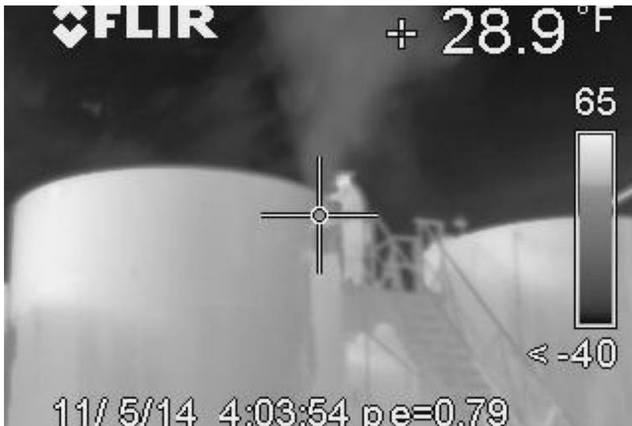
Plume of chemicals coming out of the top of a tank, taken with an infrared camera.
