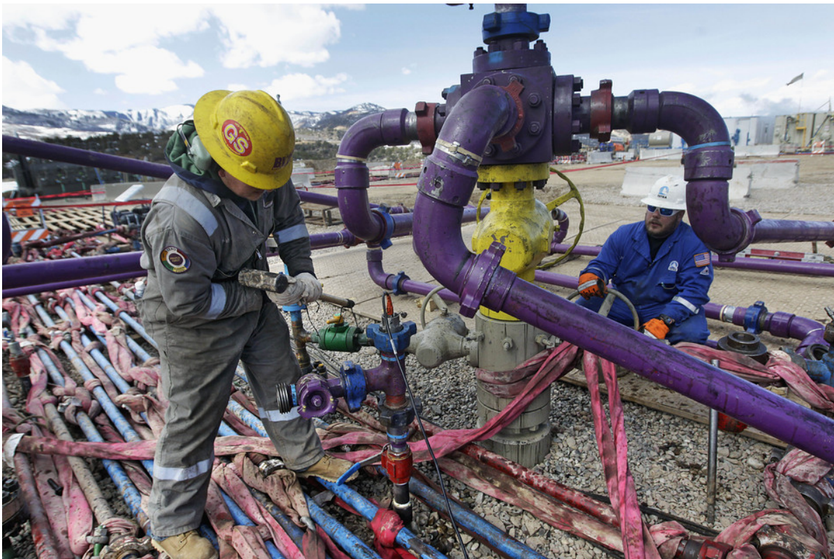
Workers tend to a well head during a hydraulic fracturing operation outside Rifle, Colo., on March 29, 2013. Increased production has driven down oil prices.
